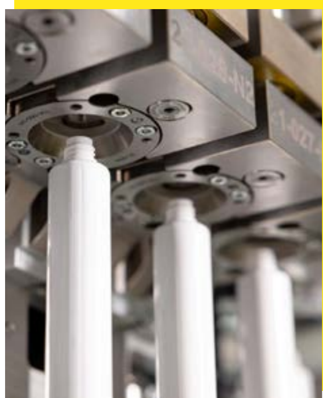
Production of PE-based mono-material tubes on PackSys machines
