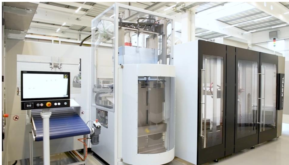
KSA modules, such as the bag inserter or carton sealer shown here, can be connected to existing and new KMD machines. © KIEFEL GmbH
